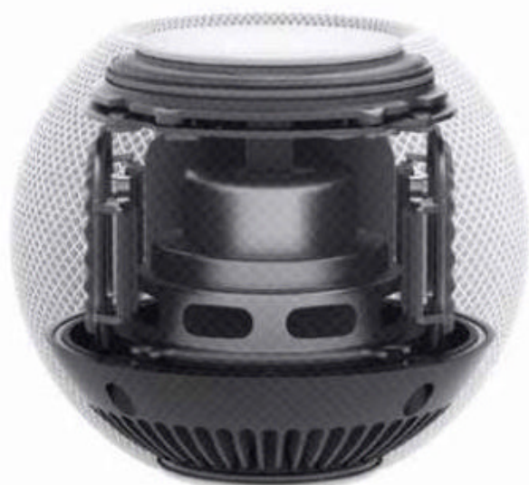
The device houses a full-range audio driver with force-cancelling passive radiators
